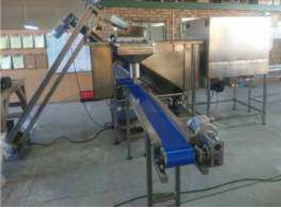
Figure 2: Elevator section of the processing line.
